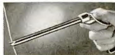
Cutter snips wires or grips articles hard to reach
